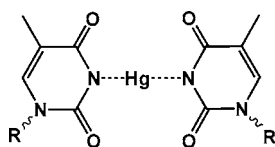
Figure 1. Structure of the thymine–Hg(II)–thymine complex.
